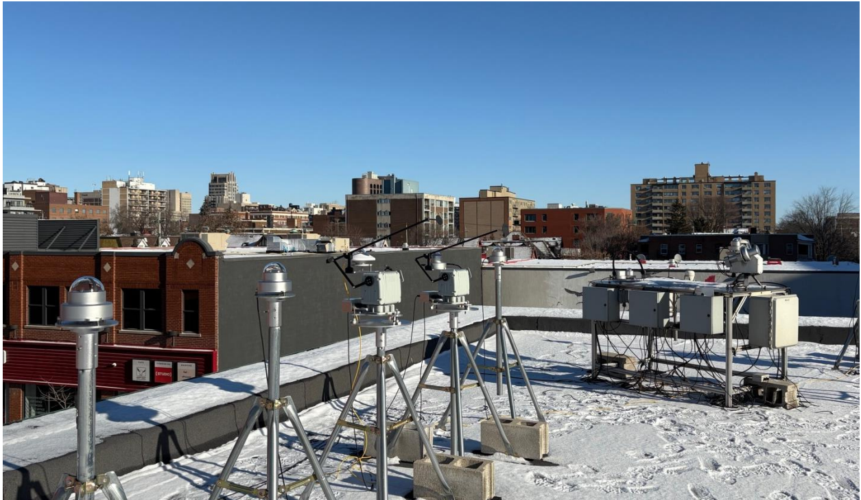
Figure 3. Spectrafy roof-top test site showing SolarBand-C3 prototypes, alongside broadband and spectral reference sensors.
