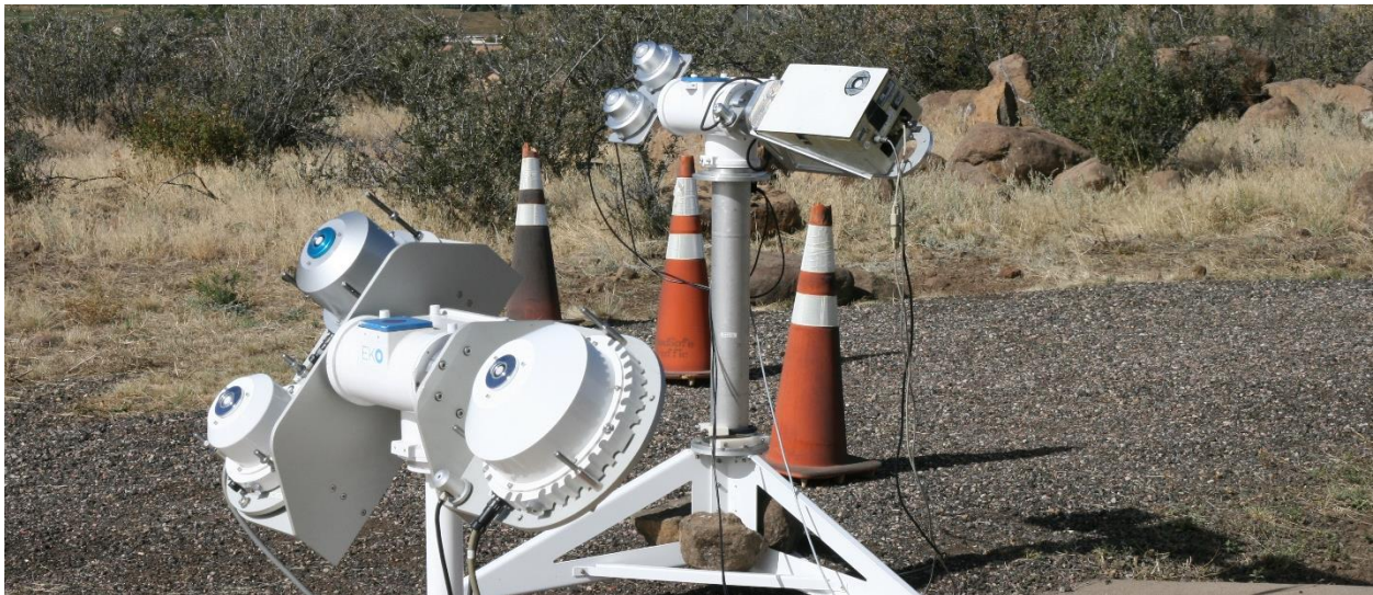
Figure 3. Calibration setup with the SolarSIM RUs and Licor 1800 spectroradiometer (background) and the EKO WISER (MS711/MS712) spectroradiometers (foreground).
