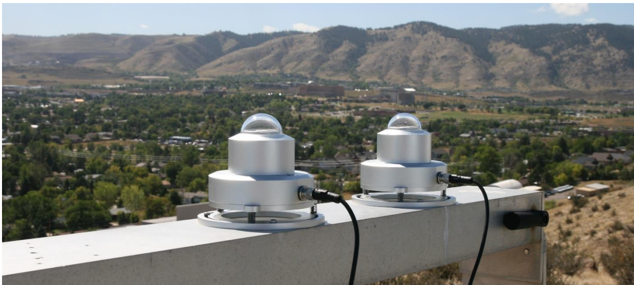
Figure 2. The SolarSIM-G/GUV reference units in operation at NREL's Solar Radiation Research Laboratory, October 2017.
